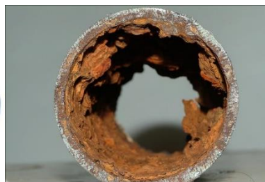
GI Pipe that has been corroded
