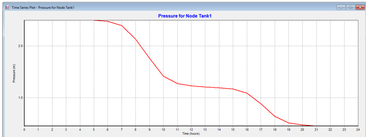
Figure 13: EPAnet Graph of Tank Pressure vs. Time
